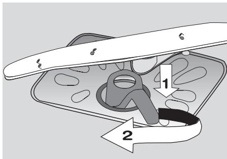
**i NEVER use the dishwasher without filters. Incorrect repositioning and fitting of the filters will produce poor washing results and will result in damage to the appliance.**
