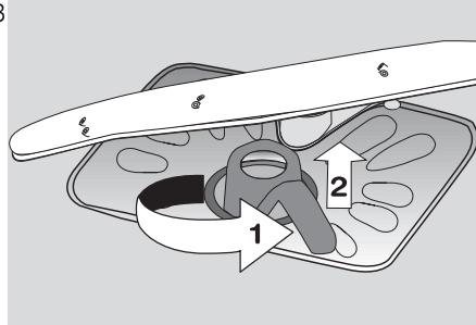
4. Take hold of the coarse filter (**A**) by the handle with the hole and remove from the microfilter (**B**).
